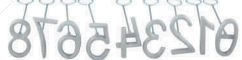
ST-01-1024 Aluminum Paint Branding Irons Made of aluminum castings, light in weight. Set consists of nine irons in 2.5" sizes. 0.5" depth, 1.5" width. Also available in 4" sizes. NOTE: A set 0-9 does not include the figure 9. The 6 iron can be reversed to make the figure 9.
