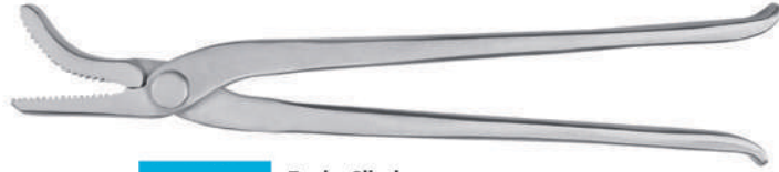
ST-01-1102 Farrier Clincher For use on high and low nails. Used to roll over nails with curved jaw. Length 13" c/s. Also available in stainless steel.
