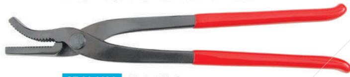
ST-01-1104 Farrier Clincher For use with larger nails used in saddle horse hoofs to roll over and clinch nails. Oil quating makes it rust resistant. Length 12" c/s. Also available in stainless steel.
